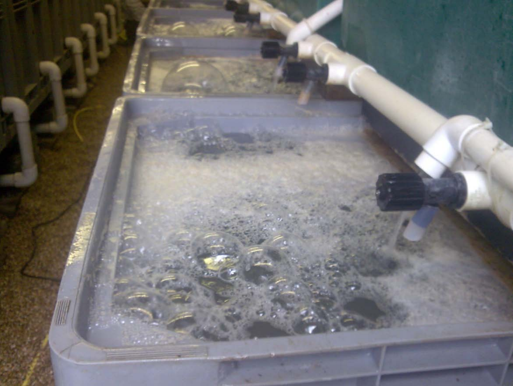
Photo 1 – Sodium hydroxide (NaOH) being circulated through recirculation systems
